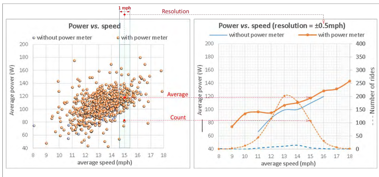
Figure 3 – Scatter and line graph presentations of the same data (751 rides; 704 with, 47 without a power meter)
